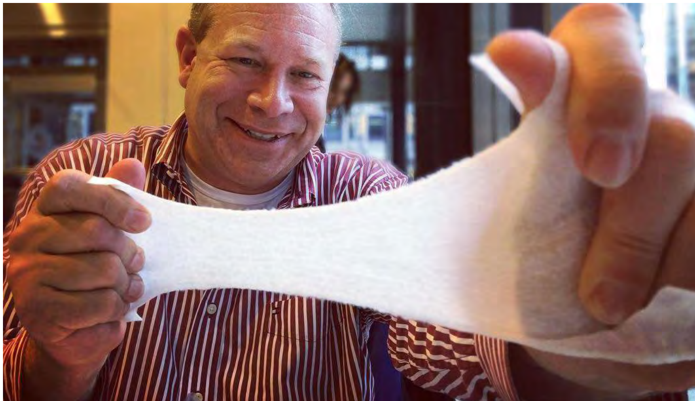
Barry Orr stress tests a “flushable wipe”.
