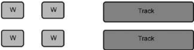
Ground contact area for wheeled versus tracked equipment
