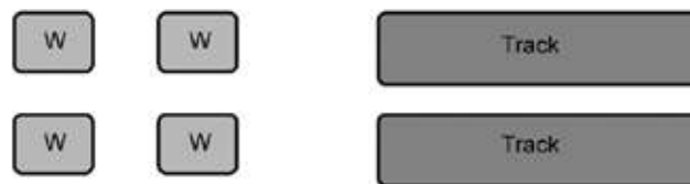
Ground contact area for wheeled versus tracked equipment
