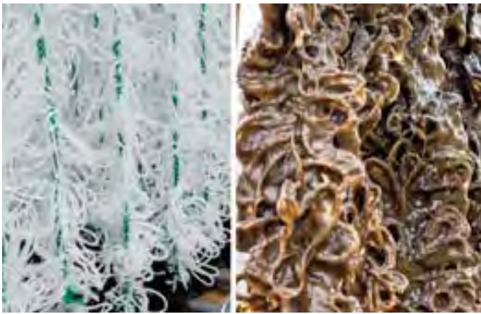
A closeup of a BioCord Reactor shows the media prior to installation (left) and after a concentrated biofilm of preferred microorganisms has been established (right).
